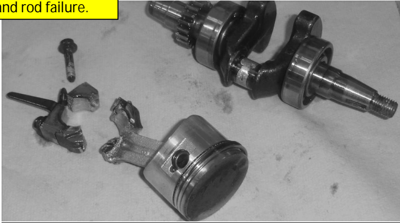
Engine crankshaft and rod failure.
